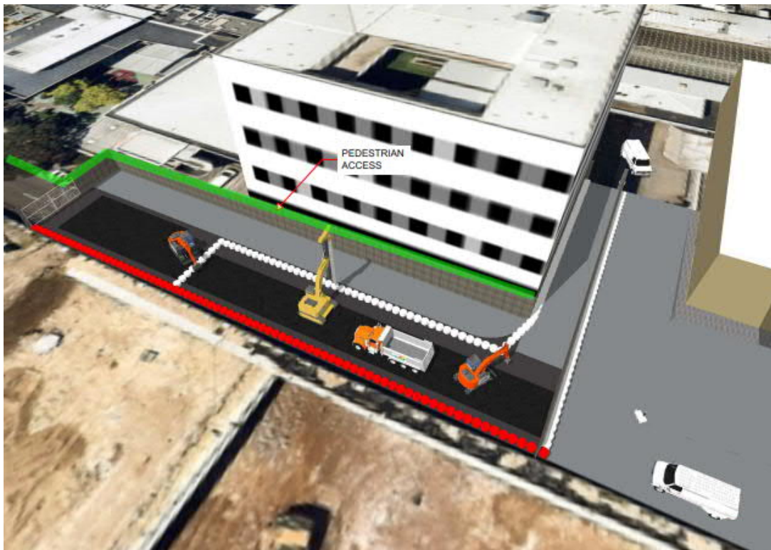
Figure 9 –North stage – retention piling – stage 3 of 6
