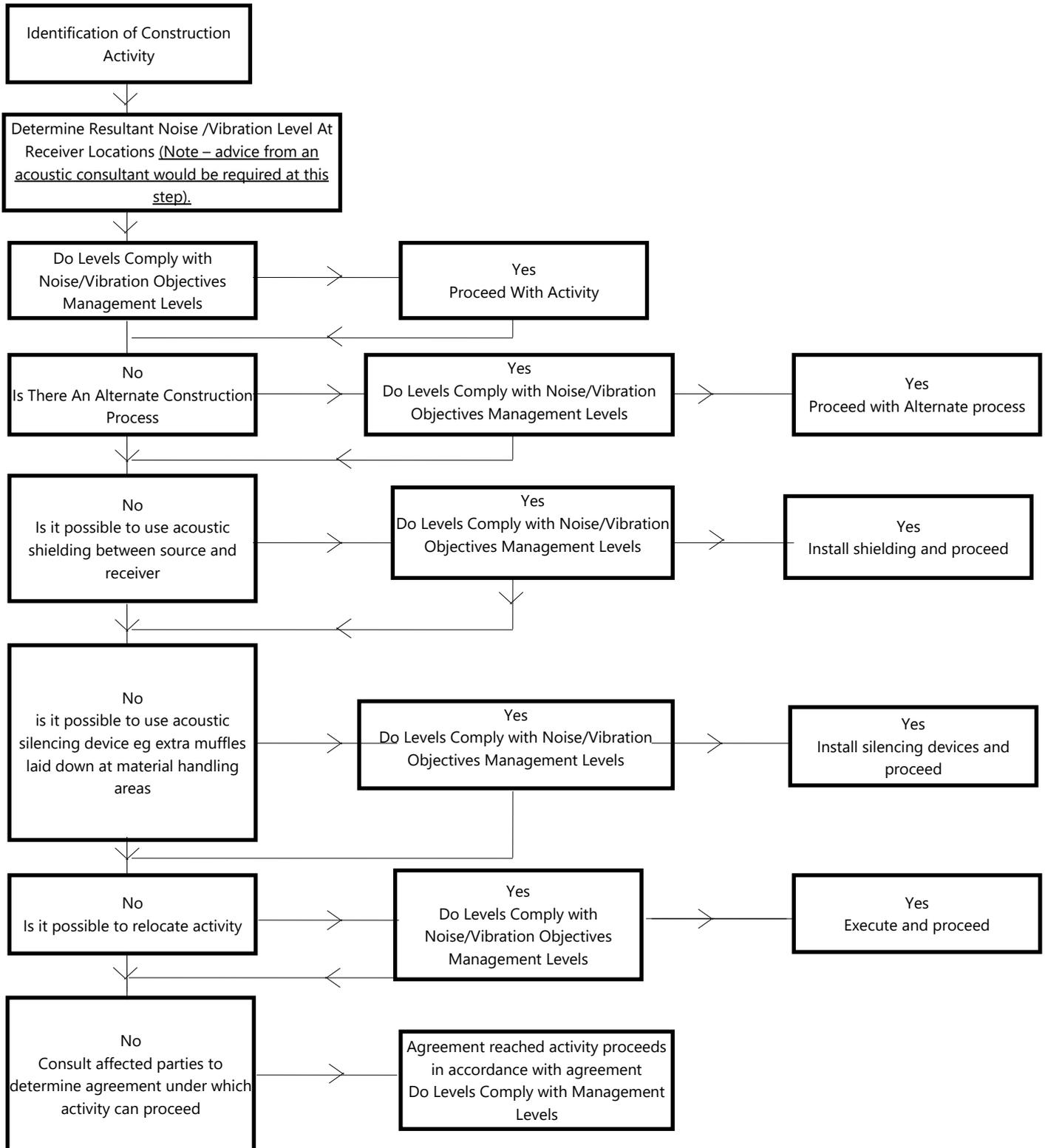
**Figure 2 – Process Flowchart**
