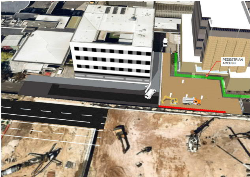
Figure 10 – South stage – Bulk excavation– stage 4 of 6
