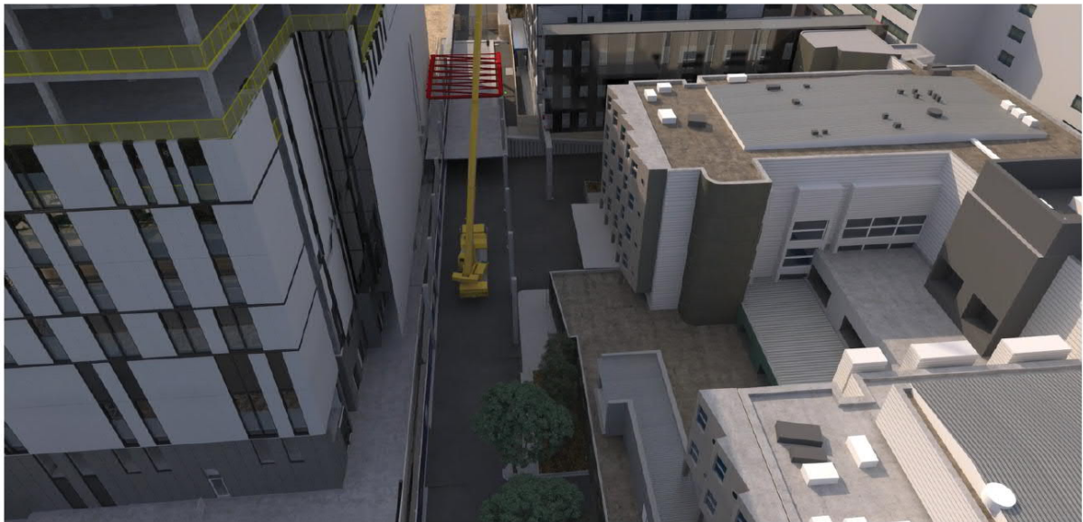
Figure 13 – Structural Steel elements supported above Hospital Road
