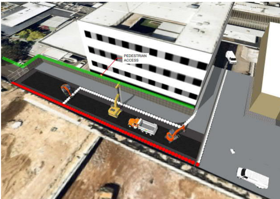
Figure 9 –North stage – retention piling – stage 3 of 6
