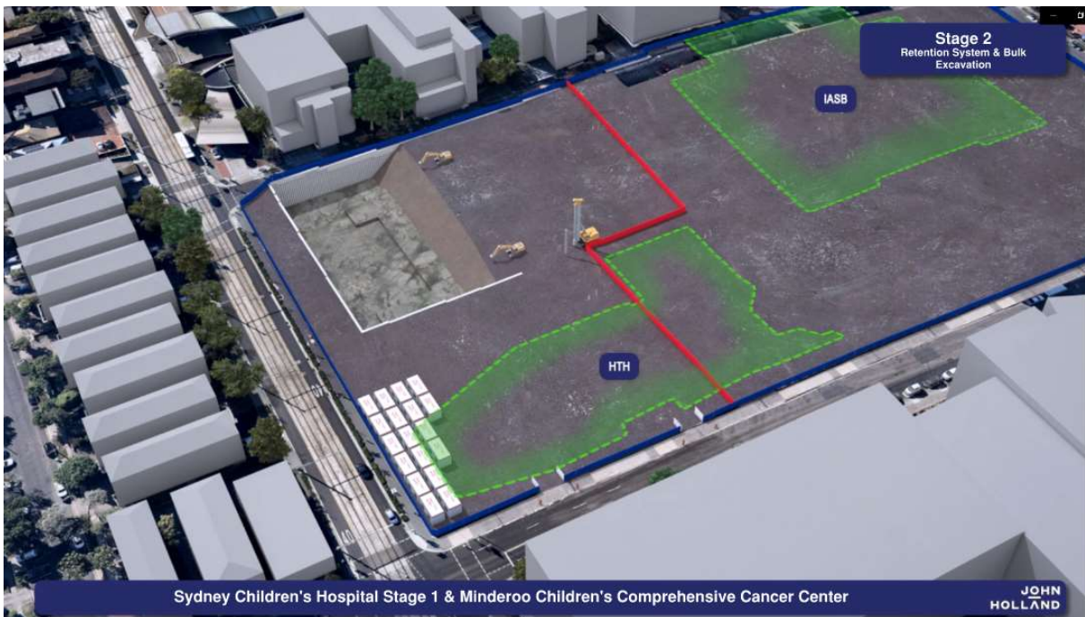
Figure 3 – Stage 2 Retention System & Bulk Excavation
